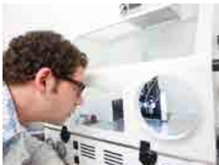
Ed uses the ultrasonic atomisation machine to coat sheets of polymer with tacrolimus
