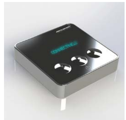
Hub for patient use to transmit live activity data for processing and feedback
